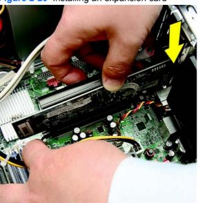
Figure 2-20 Installing an expansion card
